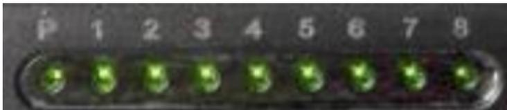
Once you've activated the Power Switch, make sure to also enable the DIP switch. The DIP switch is responsible for managing each individual antenna. Each number indicator corresponds to a specific antenna, and when the LED associated with an antenna is illuminated, it indicates that the antenna is operational.
