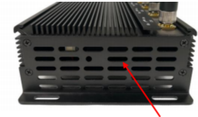
Cooling fans insided
